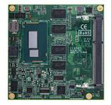
The **CEM881**, a rugged and powerful COM Express Type 6 compact module which can come with a 5th Generation Intel® Core™ i7/i5/i3 or Celeron processor®, is suitable for graphics-intensive applications such as telecommunication, medical imaging, the Internet of Things and more.
